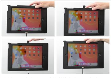
3. To insert the tablet into the power block slide the block connector into the power block. (contacts should line up) Press key lock to secure.
