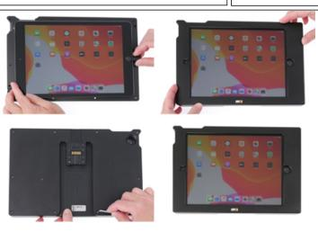
1. Place tablet face up on the Tough Sleeve back plate and connect the power cord. Fit the Tough Sleeve face plate over the tablet to enclose the device. Making sure to hold the sleeve together flip it over and secure using the enclosed screws. Once in place the tablet will be secured inside the Tough Sleeve.
